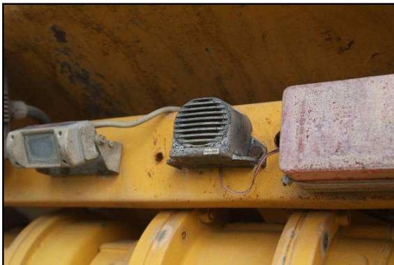
Fig 15. All mobile plant is fitted with Brigade broad band reversing alarms
