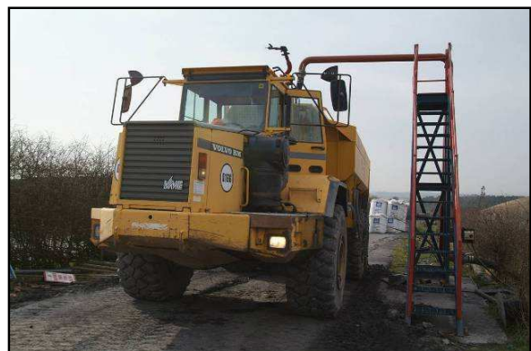
Fig 20. The filling station takes approximately 6 minutes to fill 25000 litres
