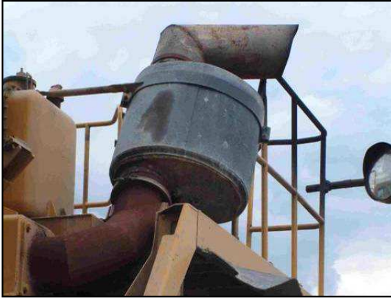
Fig 8. Standard CAT 777 exhaust silencer
