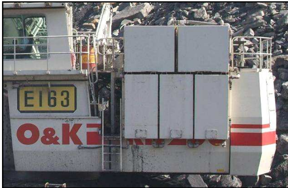
Fig 23. 10 Tanks fitted to the RH200 – total capacity 16000 litres
