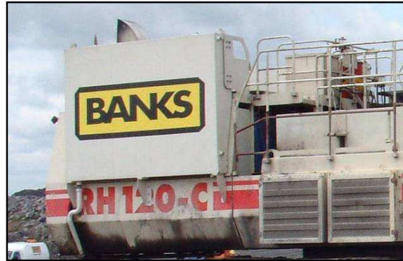
Fig 21. Terex RH120 fitted with water tanks holding approximately 6000 litres
