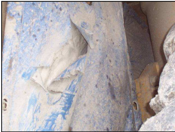
Fig 14. Damage to CAT 785 Engine side quilt
