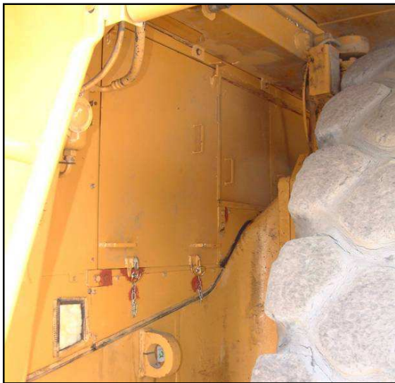
Fig 5. Acoustic panels fitted to the sides of the engine compartment on a CAT 777
