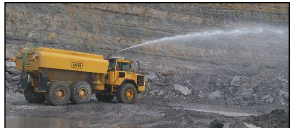
Figs 18 & 19. A Volvo A35 dump truck converted into a water tanker with two 'fishtail' sprays for wide haul roads and a water canon
