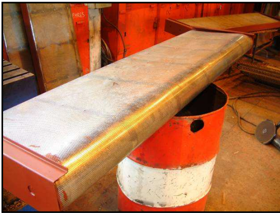
Fig 4. One of the wing sections of the splitter silencer
