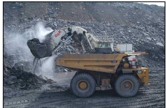
Fig 24, 25 and 26 The RH200 with dust suppression
