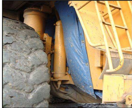
Fig 13. CAT 785 engine compartment – using quilts rather than panels and doors
