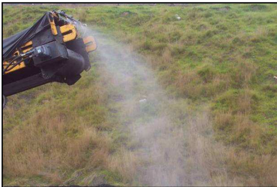
Fig 28. Fine mist sprays fitted to TESAB Coal Crusher
