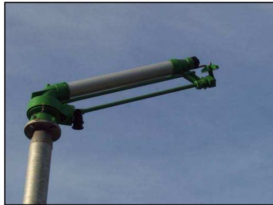
Fig 29. Polaris Rain Head gives a 65m throw
