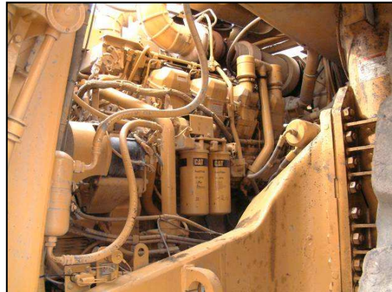
Fig 3. The open engine compartment of a CAT 777 dump truck before insulation was fitted
