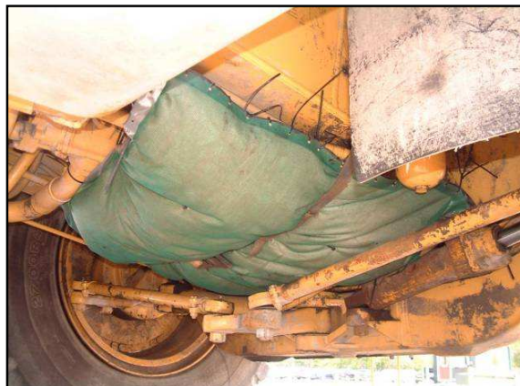
Fig 7. Prototype under body acoustic quilt – Later replaced with a fire retardant type
