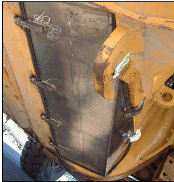
Fig 6. Engine compartment underside doors – these were later replaced with acoustic quilts
